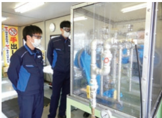
Training on experiencing the risk of leakage from flanges
